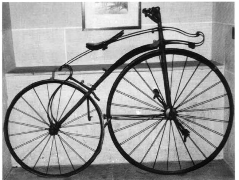
Compagnie Parisienne diagonal frame with wire wheels and suspension in Compeigne museum cl870
